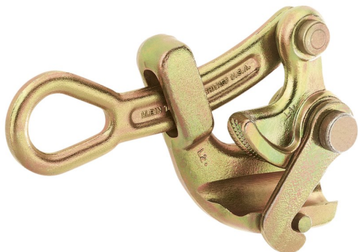
Haven's Grips #1625-20 Knurled eccentric jaw applies gripping Pressure to 1/4" of cable area. Used for Guy strand and wire rope.
